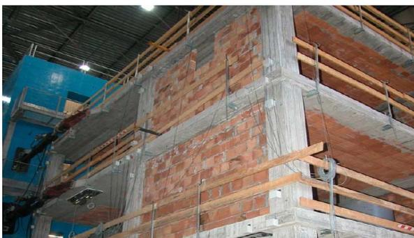
**Fig. 4: Adding infill wall**
