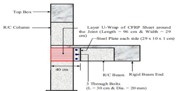
**Fig. 12: B-C joint jacketing with mechanical anchorage system**
