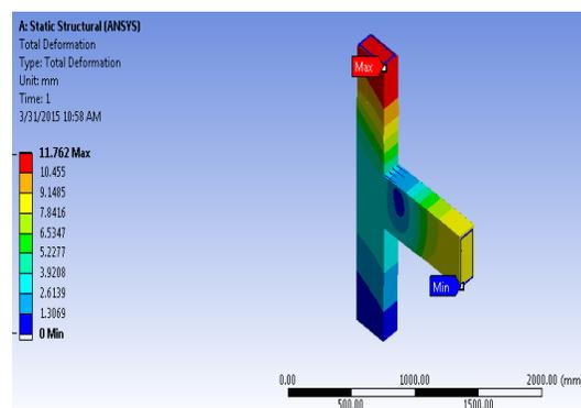
**Fig. 10: Deformation after Jacketing**
