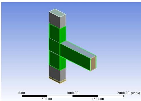
**Fig. 9: B-C joint jacketing with steel plates**
