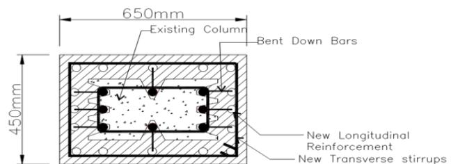
**Fig. 8: Typical Section showing Column Jacketing**
