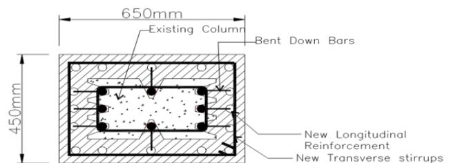
**Fig. 8: Typical Section showing Column Jacketing**
