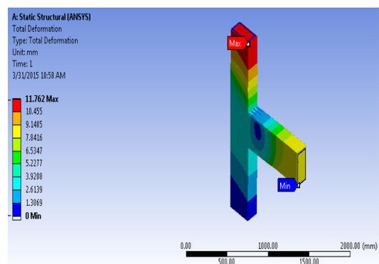
**Fig. 10: Deformation after Jacketing**
