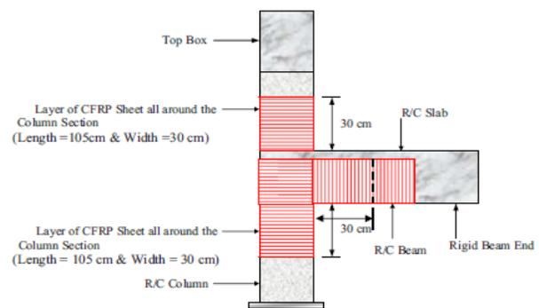
**Fig. 11: B-C joint jacketing with CFRP sheets**
